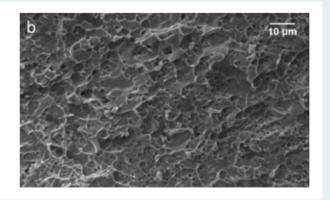
SEM image of the fracture surface of a nitinol wire, in proximity of a micro laserwelded region. The analysis of the micromorphology indicates a ductile behaviour, confirming that the adopted welding methodology preserves the mechanical characteristics of the super-elastic alloy.
