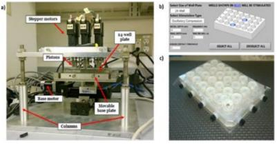
Figure 1: Hit-MACE device used to apply compressive load over cartilage plugs (a), screenshot acquired during a compressive loading experimental set-up (b), customized lid used to maintain sterile conditions during compressive cycles (c).
